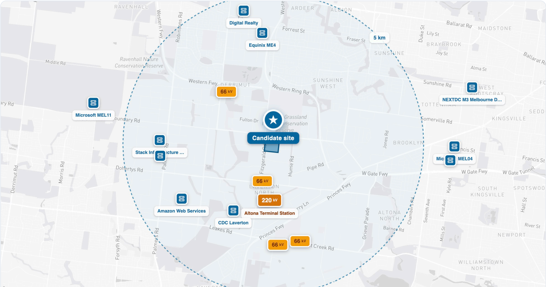
Substations (amber, with nominal voltage; the terminal station in darker amber) and existing data centres (server marks) within the 5 km ring around the candidate site.
